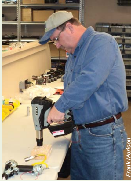
AWA's Tim Holmes tests the cordless, gas-powered TED captive bolt tool at Bock Industries.
