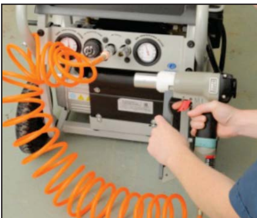
■ Zephyr-E Gun in the non-fired position with the bolt head recessed in the barrel.
